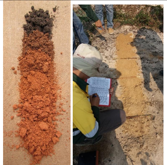
Two soil profiles obtained using an auger. The one on the left has been laid on a mat, the one on the right on cleared ground adjacent to the auger hole
